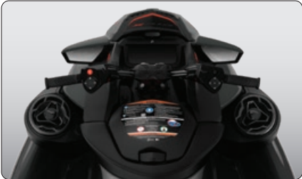
Tech Package (optional) Levels up entertainment and functionality on the water. It includes a factory-installed, truly waterproof Bluetooth® audio system, a 7.8" color display and a USB port.
